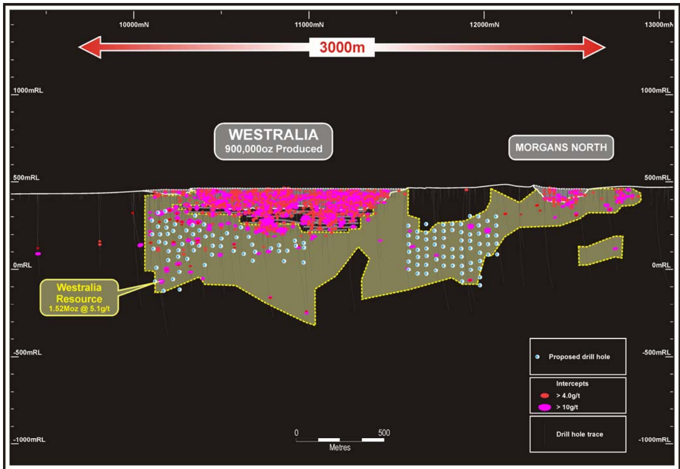
Figure 1: Planned drilling program over the Westralia Prospect with 62 diamond drill holes planned for potential Westralia Underground (blue dots on left hand side of image) and 67 diamond drill holes planned for potential Morgans Underground (blue dots on right hand side of image).
